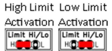
GRBL default is for limit switch activation through a normally-open switch connecting the limit switch pin to ground. This mode is picked by using the Limit Hi/Lo jumper to select the center and right points. If you prefer to have high activated limit switches, use the Limit Hi/Lo jumper to select the center and left pins.
